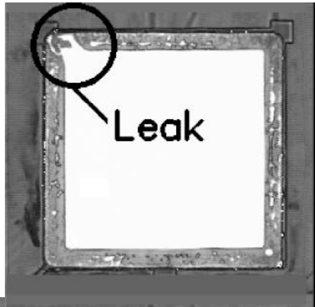
Figures 14 & 15: Kovar lids soldered to ceramic packages. Notice the voids, white regions, within the solder seal areas of both packages. The circle indicates the location of a seal leak.
