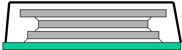
Figure 1: Diagram of a stacked die package containing two die of different sizes and a silicon spacer.
