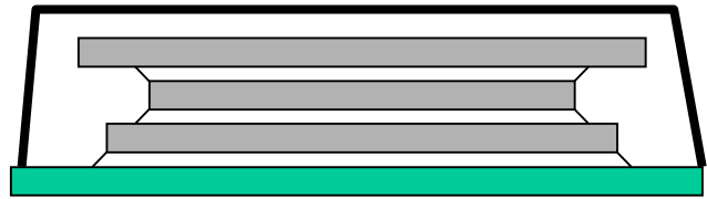
Figure 1: Diagram of a stacked die package containing two die of different sizes and a silicon spacer.
